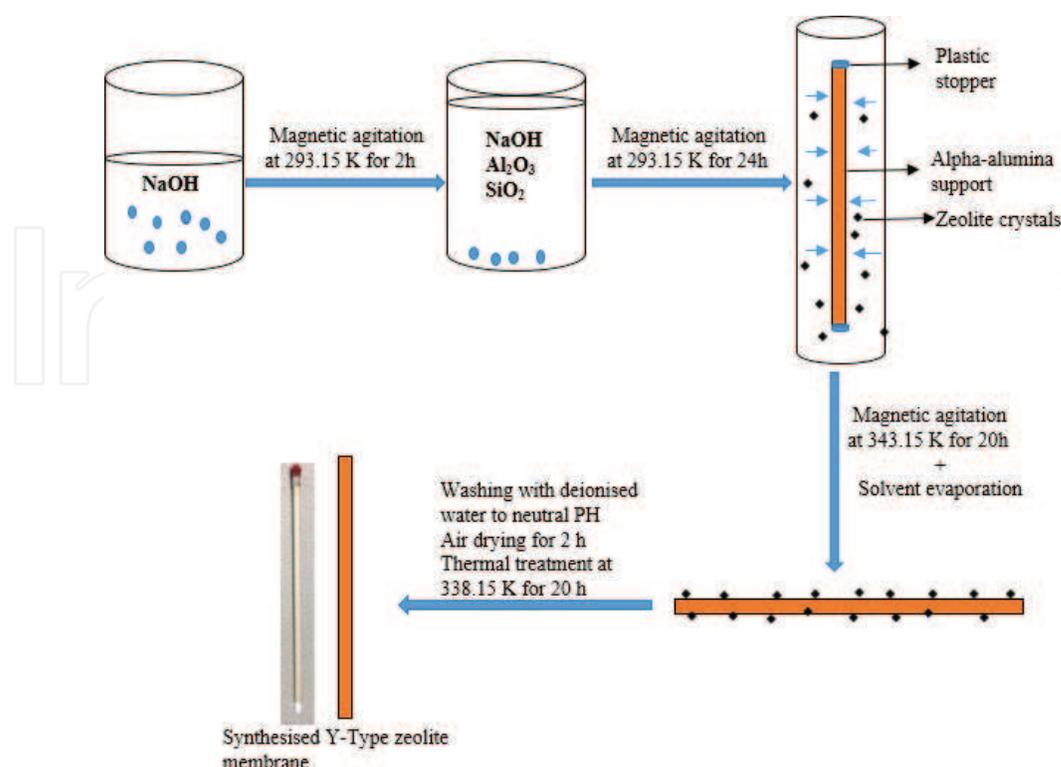
**Figure 1.** Schematic of the solid-state crystallisation route for y-type zeolite synthesis.
