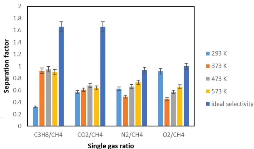
Figure 8. Separation factor of gases with increasing temperature.
