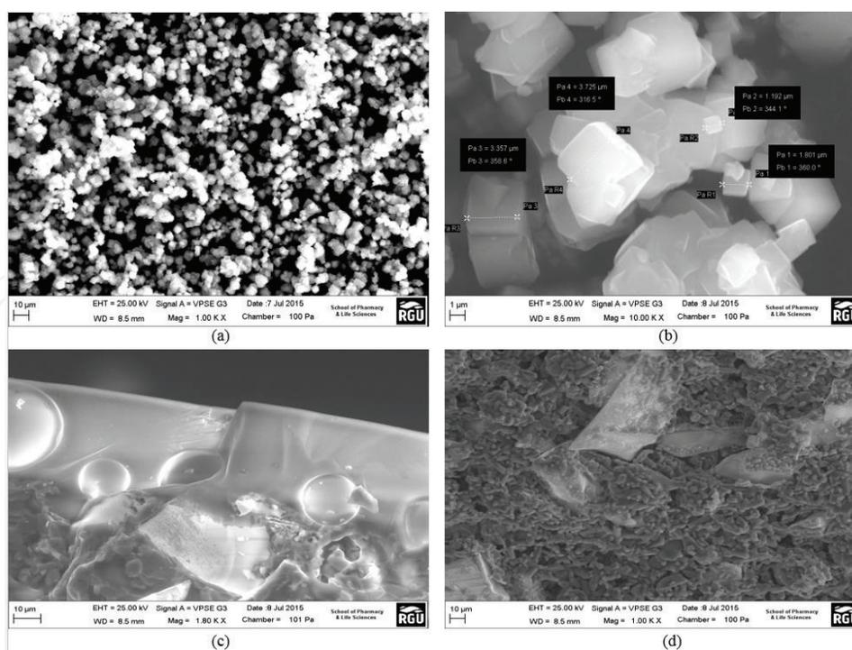
**Figure 2.** SEM of the zeolite particle samples at (a) before deposition (b) higher magnification before deposition (c) alumina support (d) 24 h crystallisation.
