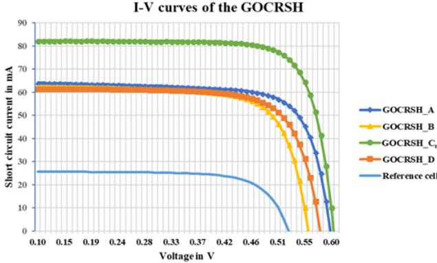
Fig. 3. I-V curves of the GOCRSH under STC conditions at normal incidence
