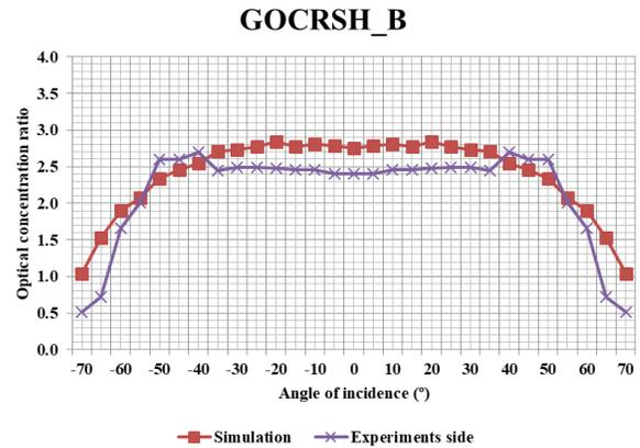
Fig. 6. Experimental and simulated angular acceptance of the GOCRSH\_B
