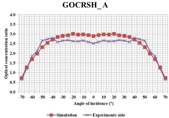
Fig. 5. Experimental and simulated angular acceptance of the GOCRSH\_A
