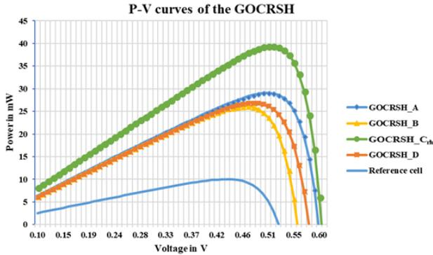
Fig. 4. P-V curves of the GOCRSH under STC conditions at normal incidence
