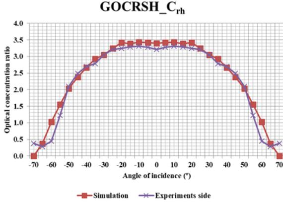
Fig. 7. Experimental and simulated angular acceptance of the GOCRSH\_C<sub>rh</sub>
