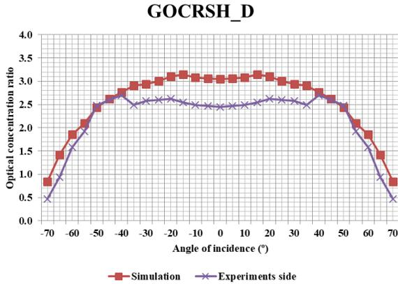
Fig. 8. Experimental and simulated angular acceptance of the GOCRSH\_D
