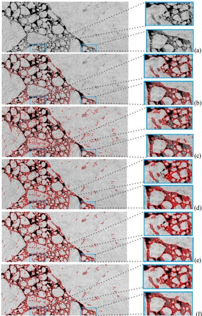
Fig. 9. Comparison of segmentation results with GT image. (a) Original sea ice image. (b) GT image. (c) Result of  $K$ -means + HMRF-EM. (d) Result of General SLIC. (e) Result of RPCA+ General SLIC. (f) Result of proposed method.
