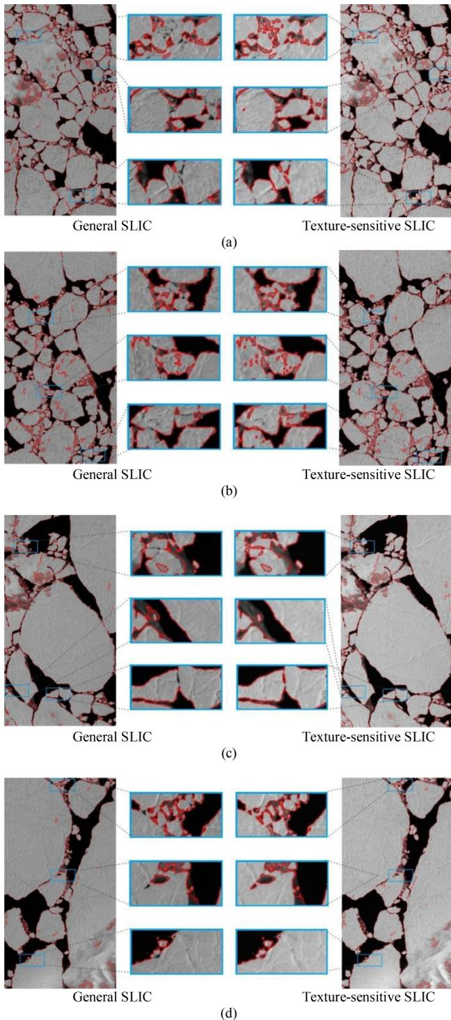
Fig. 6. Visual comparison of segmentation results. (a) Comparison of top-left image. (b) Comparison of top-right image. (c) Comparison of bottom-left image. (d) Comparison of bottom-right image.
