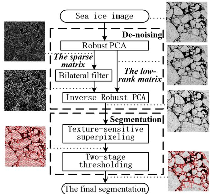
Fig. 1. Flowchart of proposed algorithm for sea ice floe segmentation.
