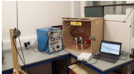
Fig.4. The experimental set up: A floating-electrode PD emulator is used as a PD source [16].
