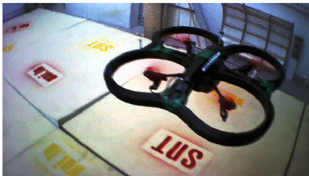
Fig. 17 Visual tracking of quadrotor from camera-equipped quadrotor
