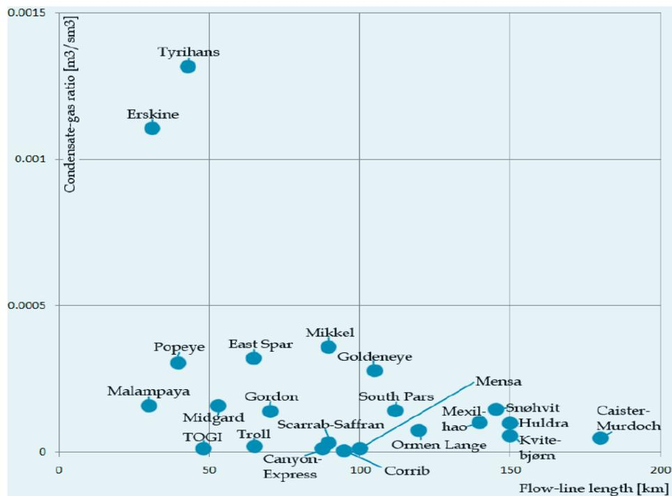
Figure 1-3: Multiphase flowline projects-completed and planned (9)
