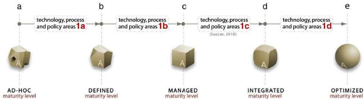
Figure 2.5: BIM Maturity Levels at BIM Stage 1 (Succar et al. 2013)
