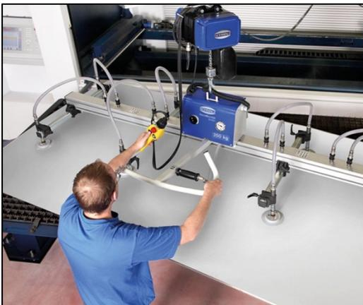
Figure 20. Suction cup lifting equipment.
