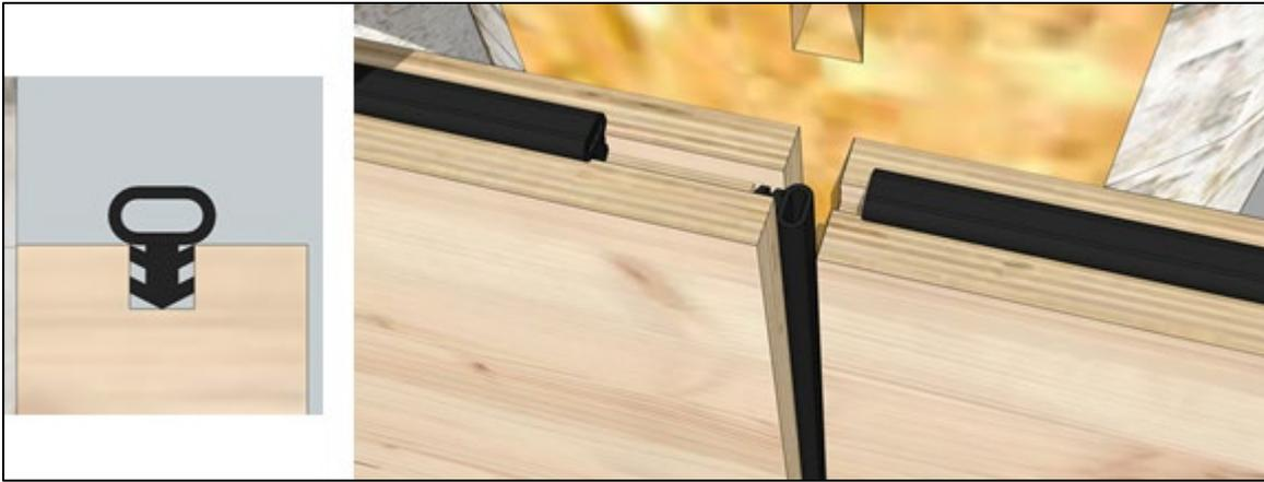
Figure 15. Dry Elastomer seals.
