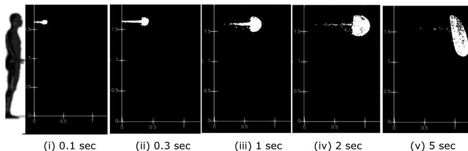
FIG. 4. Saliva aerosol transports due to continuous coughing and breathing. Multimedia view: <https://doi.org/10.1063/5.0042952.2>
