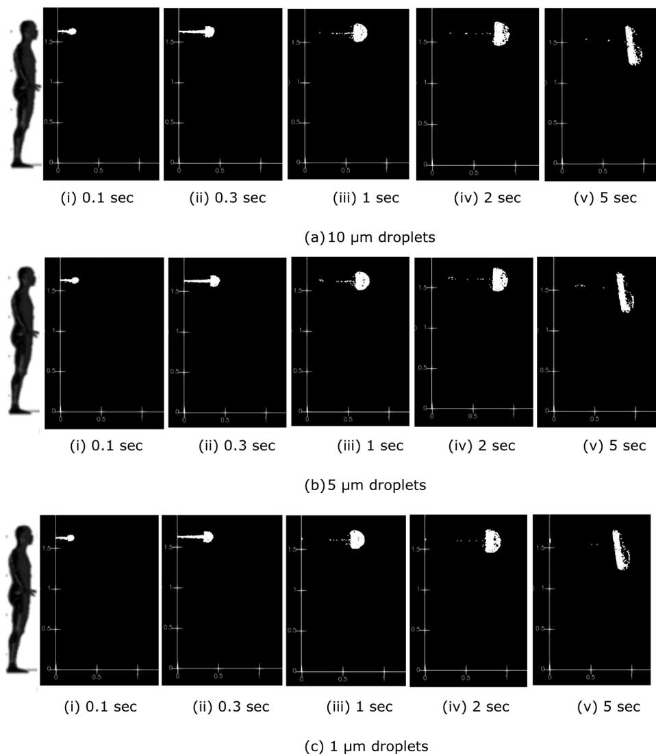
**FIG. 2.** Saliva aerosol trajectories from a single cough: (a)  $10\ \mu\text{m}$  droplets, (b)  $5\ \mu\text{m}$  droplets, and (c)  $1\ \mu\text{m}$  droplets. Multimedia view: <https://doi.org/10.1063/5.0042952.1>
