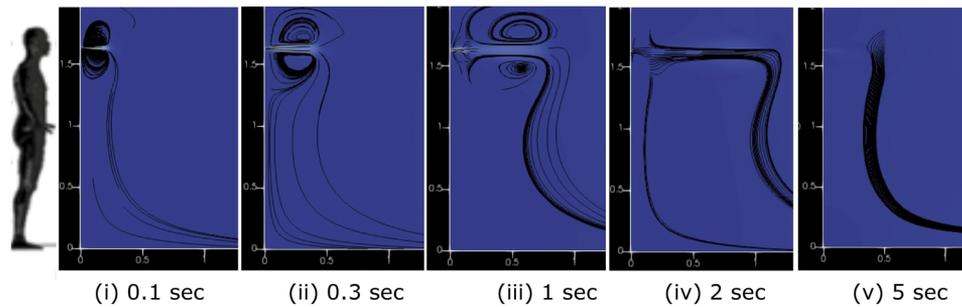
FIG. 5. Air velocity in the longitudinal direction for continuous coughing and breathing with streamlines.
