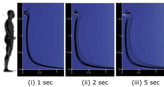
FIG. 9. Air velocity during breathing with streamlines.
