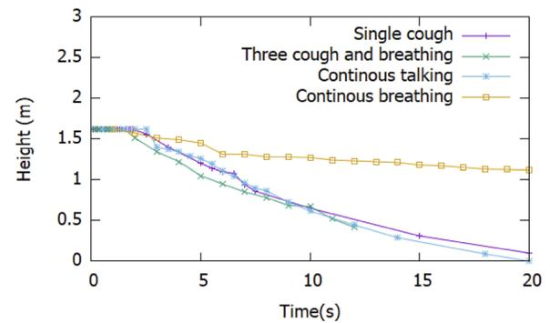
FIG. 11. Fall rate of aerosol cloud.
