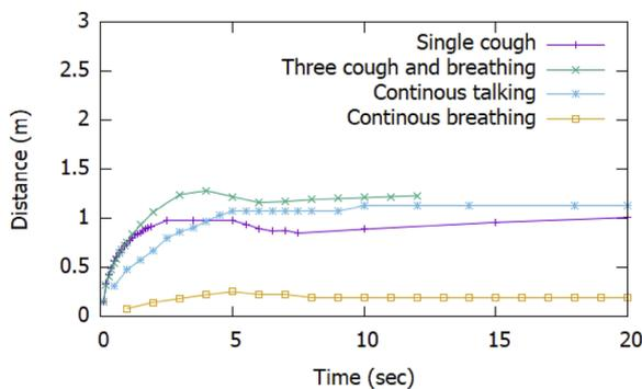
FIG. 10. Aerosol cloud penetration distance.
