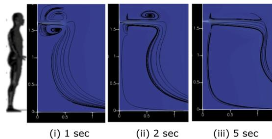
FIG. 7. Air velocity during continuous talking with streamlines.
