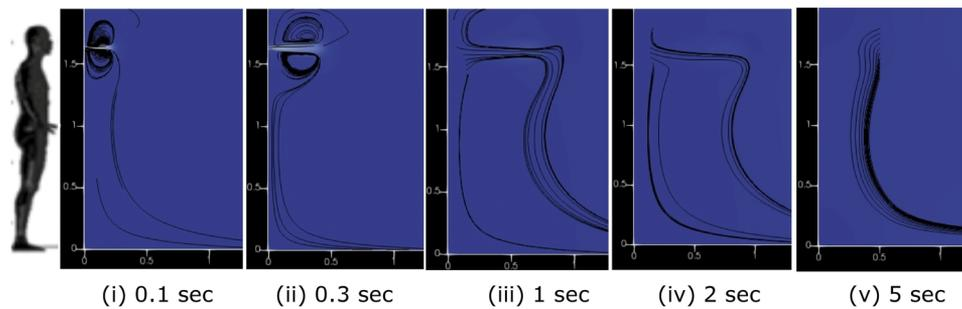
FIG. 3. Air velocity in the longitudinal direction from a single cough with streamlines.
