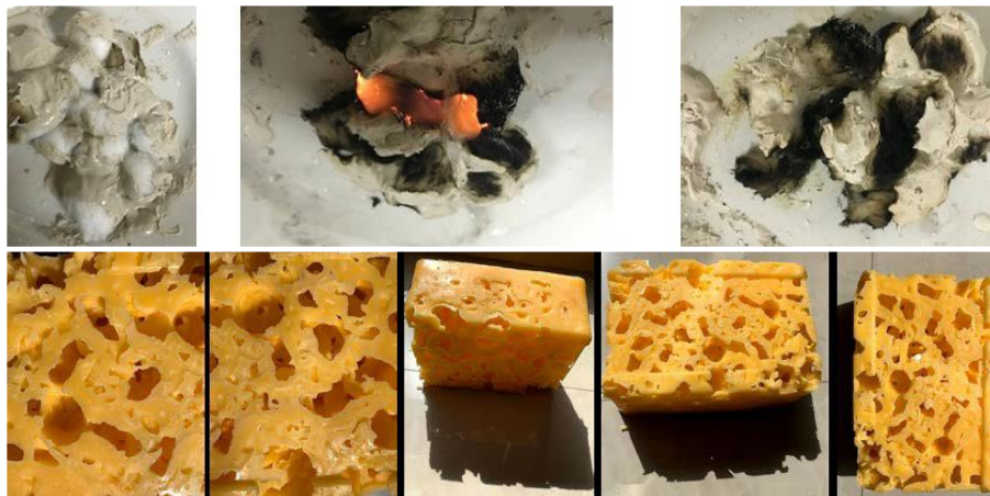
Figure 7. Examples of unique experimentation with formwork used for casting materials, including using cotton while applying heat to the casted material, as well as using ice cubes as formwork for casting hot wax. [Photo credit: Reem Shahin, Mariam Ibrahim]
