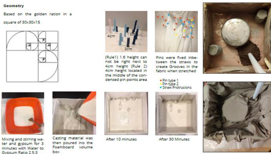
Figure 3. Example student setup of the formwork for their material exploration phase. [Photo credit: Yasmin Hazem]
