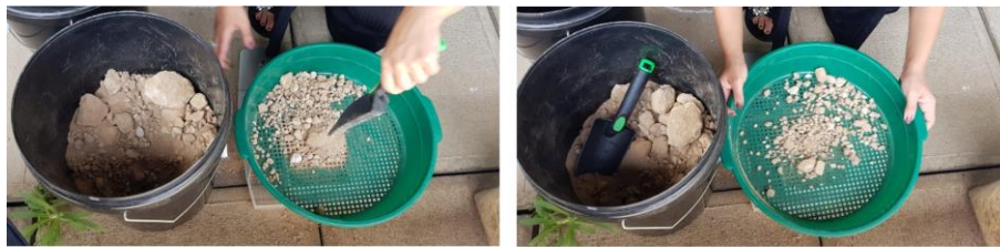
Figure 3. Soil sample sieved to remove large stones.
