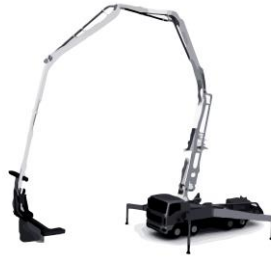
Figure 5. A mobile concrete pump used as a concrete 3D printer
