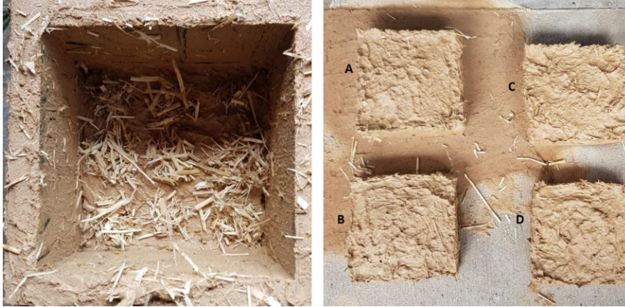
Figure 10. (left): Mud block C: straw pocketing; (right): Mud block A- the control that has no straw density grid layer; Mud block B- 1 layer of the straw density grid using medium length fibers at 1/2; Mud block C- 1 layer of the straw density grid using short length fibers at 1/2; Mud block D- 2 layers of straw using short fibers at 1/3 and 2/3.
