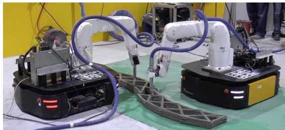
Figure 6. Swarm robotic experiment by the Singapore Centre for 3D Printing
