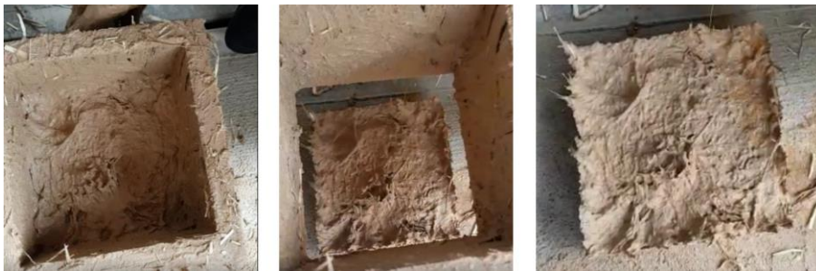
Figure 7. (left): Filling the mud mixture into the mould at only half the height of the mould; (middle): removing the filled mould; (right): the mixture holding form.
