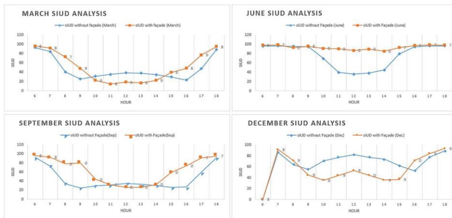
Figure 6. Comparison diagrams of sIUD index in the baseline model and research model.
