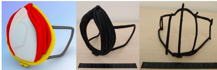
Figure 9. Virtual and real 3D model using Gravity Sketch (left and center); Freehand 3D sketch from Hyve-3D (right).
