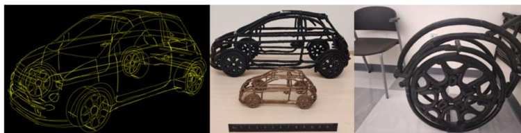
Figure 7. Freehand 3D sketches in Hyve-3D (3D vectors) (time spent: 4 hours) (left), Printed freehand 3D sketches of the car at 1/10, 1/100 (center), 1/1 scale “partial” (right).
