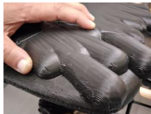
Figure 10. Aesthetic effect of 3D printed hatches for surface filling (seat of Flamingo chair).
