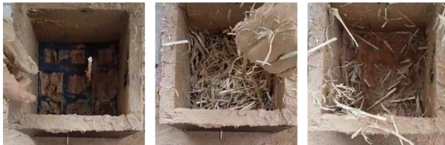
Figure 8. (left): Mud block B: square grid template at halfway (after 2 handfuls); (middle): removing the square grid template after placing straw; (right): the straw too long and not falling in the square pockets of the density grid.
