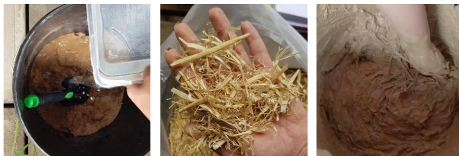
Figure 5. (left): water added to dry mix; (middle): varied straw length; (right): hand mixing.
