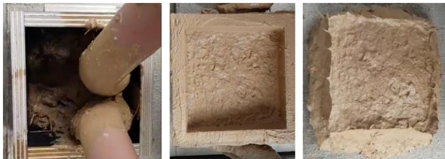
Figure 6. (left): Filling and poking the mud mixture into the mould for mud block A (control); (middle): removing the filled mould; (right): mixture slumping, not holding form.
