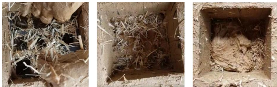
Figure 9. (left): Mud block C: square grid template being placed halfway; (middle): varied square pockets of straw after template removal; (right): mud layer on top of straw placement.
