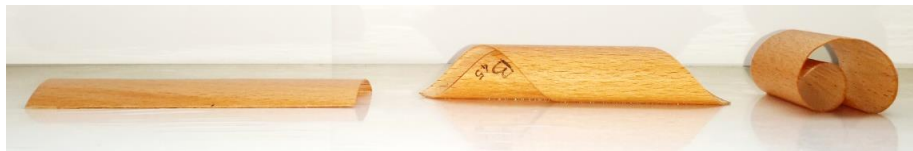
Figure 1. The response of Beech veneer samples with different grain orientations to increase in humidity (from left to right: 90° grain orientation, 45° grain orientation and 0° grain orientation) (Abdelmohsen et al., 2019a)
