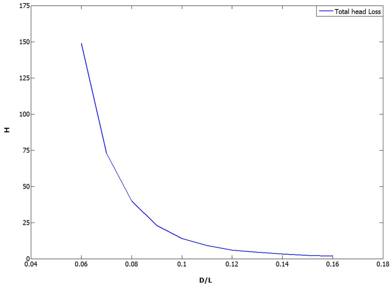
**Figure 1.** Variation of total head loss in a cylindrical capsule carrying hydraulic pipeline for a solid throughput of 50 kg/sec, or  $Q_c=0.05 \text{ m}^3/\text{sec}$ , for capsule to pipe diameter ratio of  $b = 0.8$ .
