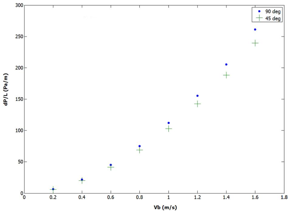
**Figure 2.** Variations in Pressure Drop in Hydraulic Bends.
