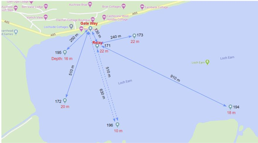
Figure 4.2: Network topology - top view; sensor nodes positions, MAC addresses and the acoustic links (arrows) marked on Google map of Loch Earn field experiments. The depth of each sensor node is shown in red. The two dashed lines show two different topologies.
