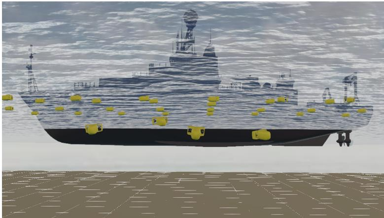
Figure 4.4: Underwater Webots simulation scene of 50 AUVs deployment, the USBL transceiver is hull-mounted on the deployment vessel.
