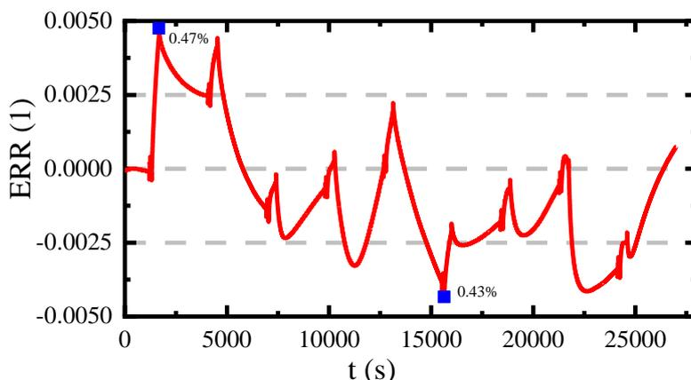
**Figure 3.** CKF-based Lithium-ion battery SOC estimation effect
