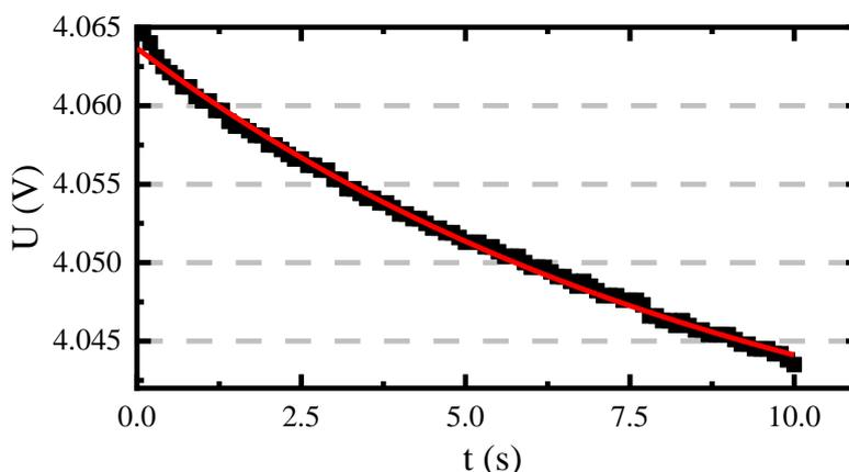
**Figure 5.** zero state response curve for SOC=1
