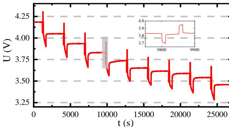
**Figure 1.** HPPC voltage curve
