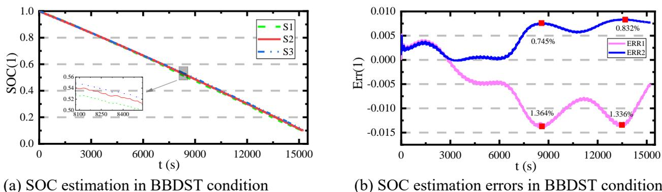
**Figure 4.** SVM-CKF-based Lithium-ion battery SOC estimation effect in BBDST condition
