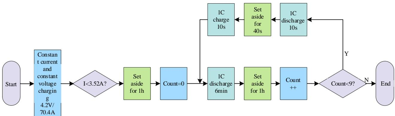
Figure 3. HPPC experimental procedure
