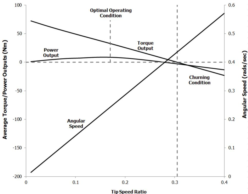
**Figure 6. Optimal operating condition of the VAMCT.**
