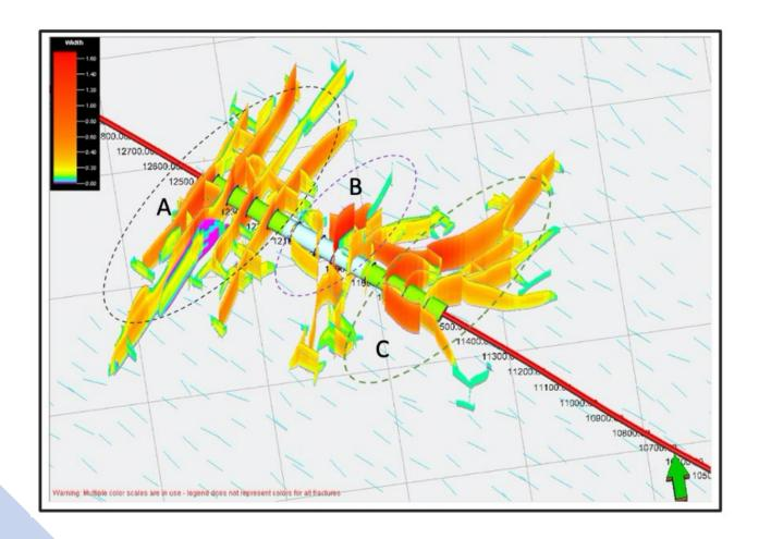
Hydraulic fracture network generated during first treatment stage, (b) Hydraulic fracture network developed during first and second treatment stage, and (c) Hydraulic fracture network generated during third treatment stage (Modified after Yew and Weng 2015)
