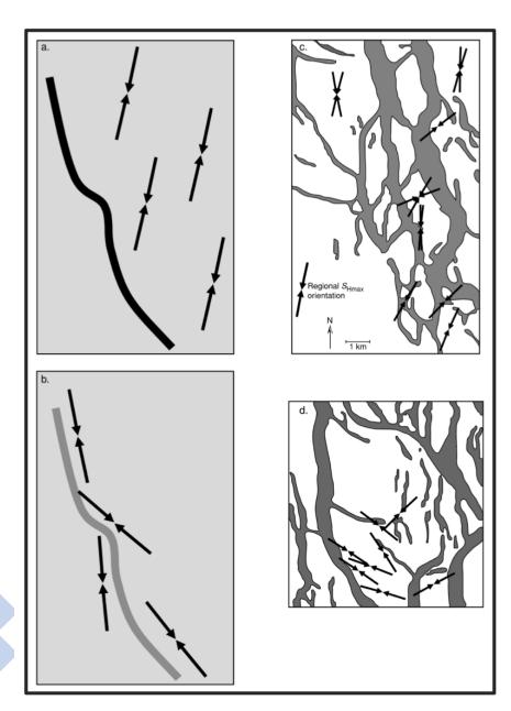
Horizontal stress rotation (a and b conceptual model before and after production respectively-Zoback 2007) (c and d from Arcabuz–Culebra field in Mexico - before and after production respectively Wolhart et al. 2000)
