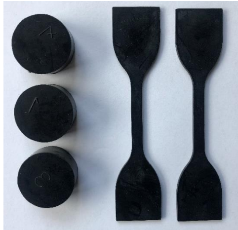
Figure 2- Unaged Compression buttons and tensile dumbbells before testing- Diameter of 29.5 mm and a thickness of 12.5 mm. Tensile dumbbells size I according to the standard with a thickness of 2 mm.
