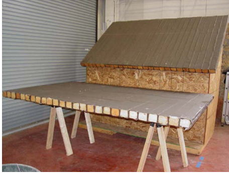
FIGURE 14: Biobased composite roof panels; one of them is mounted on a demonstration house made of timber [184].
