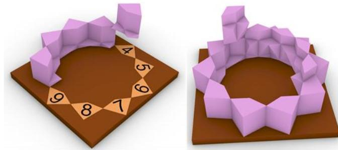
*Figure 9.* The border of the first row's components would be drawn on a board and programmed drone will put the first set of components on relevant units. Then, the components will be put on above each other, row by row.
