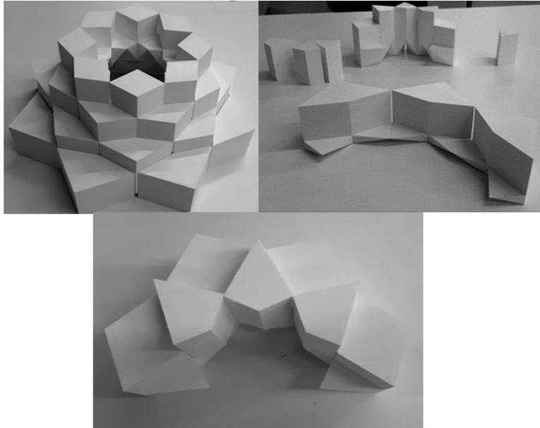
*Figure 11 The modules have been 3d-printed under 1/3 scale to test the structure resistance and have been assembled.*
