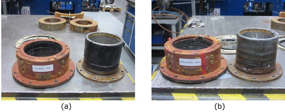
Figure 16: Simplex seals and associated liners prior to wear inspection (a) aligned (b) misaligned.
