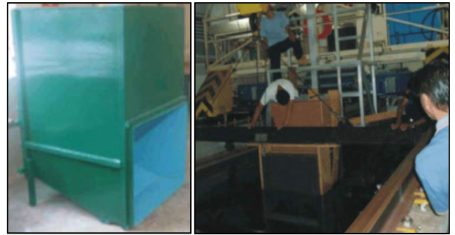
FIGURE 10. OWC lab-scale model with the savonius turbine constructed in Universiti Teknologi Malaysia (UTM) (Left), (b) OWC WEC device experimental testing in UTM towing tank (Right) [84].
