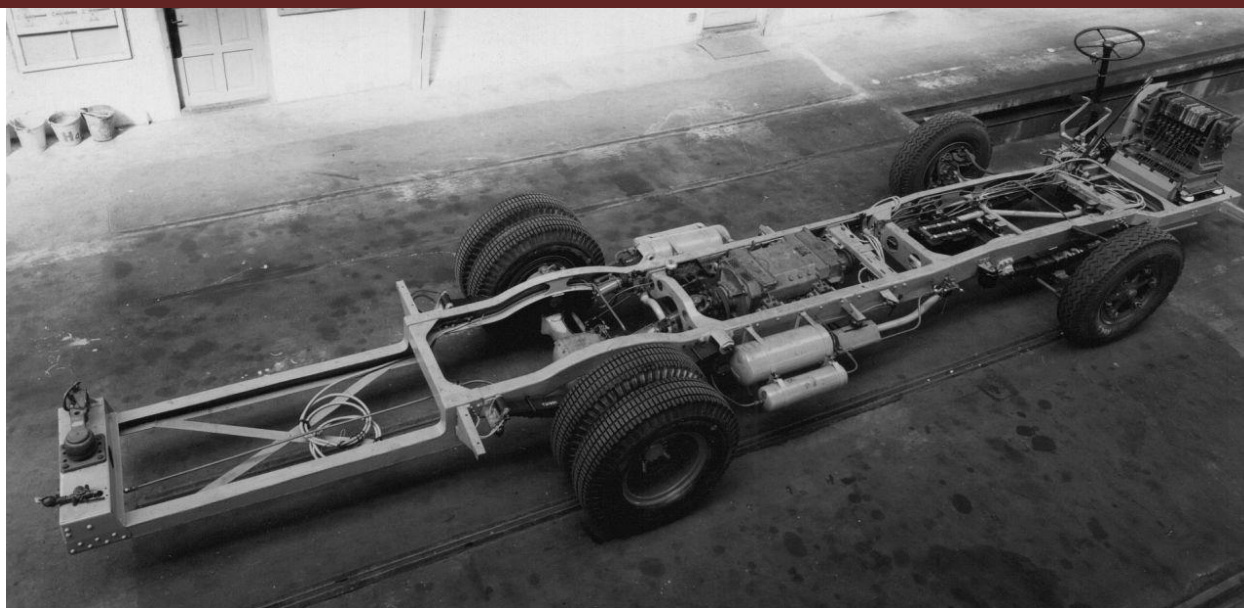
Figure 1. MAN MPE I standard trolleybus chassis, the 1940s model. The wheelbase is 4.25m, which is 1m less than in the early cars of the 1938 model. Also, early trolleybuses (Chernivtsi, Zwickau) had a rear axle single-tire wheel (in the photo – a classic double-tire wheel) (Kiebler, Ronald, 2000a).
