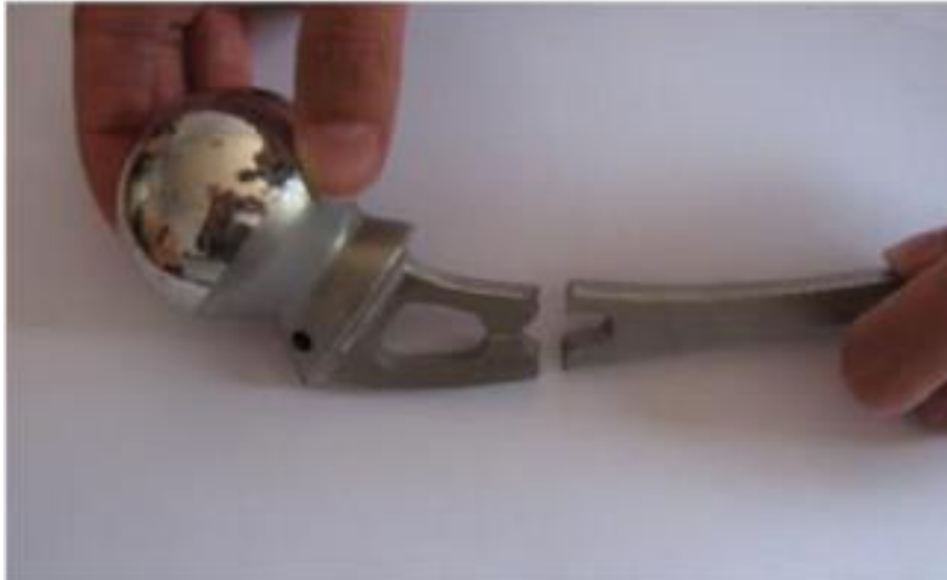
Figure 7 Failure of an artificial hip prosthesis [53].
