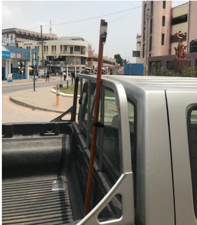
Fig 9 Vehicle-mounted weather sensor used for mobile survey in pilot study (Author generated)
