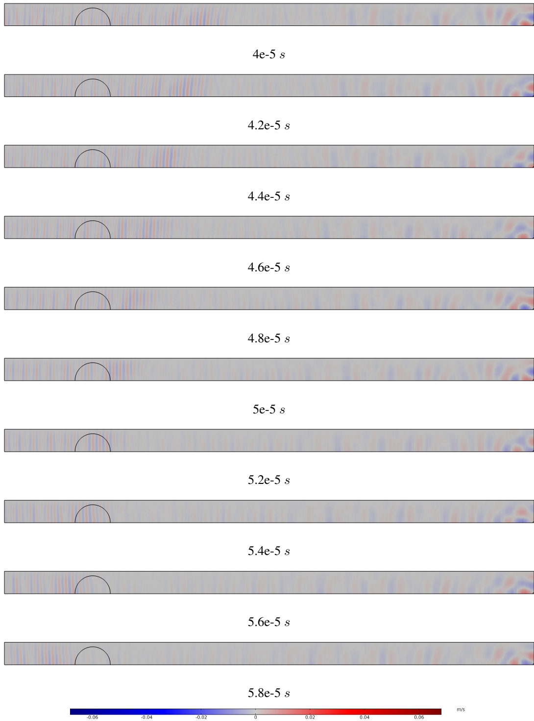
Figure 5.8: (contd.) Wave-propagation in a single 1mm aluminium adherend from an out-of-plane PLB source
