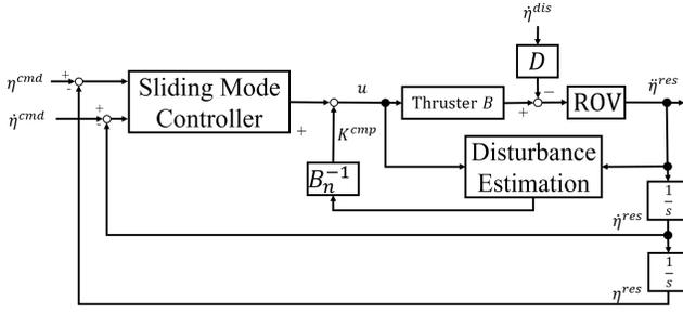
Fig. 6. Block diagram of proposed controller
