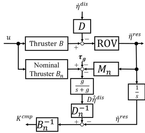
Fig. 5. Block diagram of disturbance estimation
