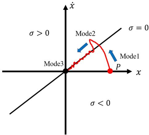
Fig. 3. Concept of sliding mode control
