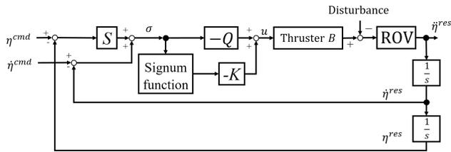
Fig. 4. Block diagram of sliding mode control
