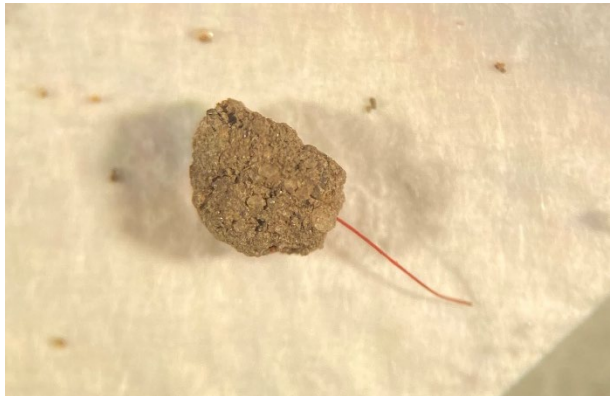
814 Figure S1. Photograph of a red fibre (identified predominantly as polyester by FTIR) partially 815 embedded in a soil aggregate under the stereomicroscope recovered from the Glensaugh 816 sample using the developed HGMS method.
