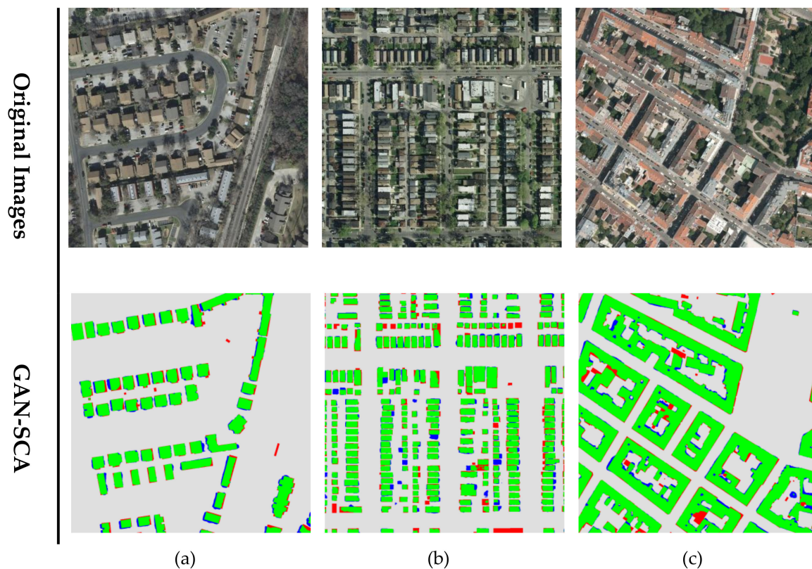
Figure 6. Building extraction results of Inria aerial image labeling dataset. (a) Image patch over Austin; (b) Image patch over Chicago; (c) Image patch over Vienna. Green: true positive (tp) pixels; Gray: true negative (tn) pixels; Blue: false positive (fp) pixels; Red: false negative (fn) pixels.
