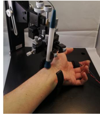
FIGURE 4. The 3D printed fixture to hold the wrist (on right) and acquisition scenario (left).
