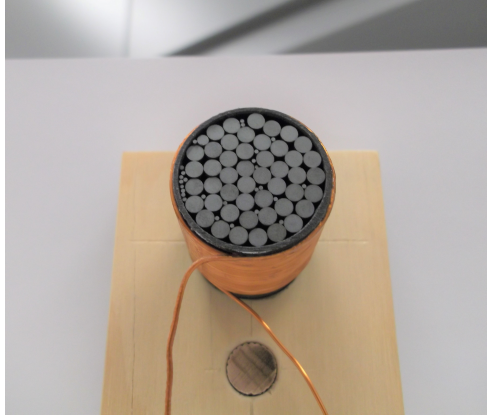
Figure 5.3: Physical structure of the employed ferrite-cored coils.
