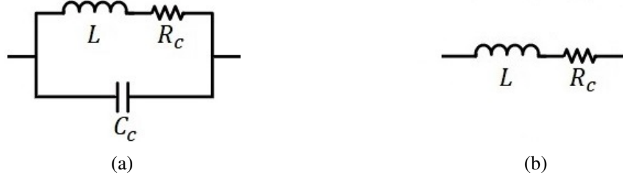
Figure 3.2: The equivalent circuit models for a typical wire-wound air-cored coil: (a) RLC equivalent model, (b) series equivalent model.
