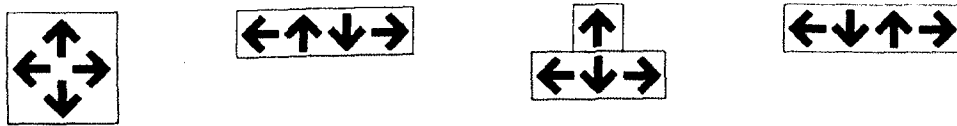
Figure 2-20: Four possible graphic combinations of arrow-key mappings for users to test which is the most natural (source: Preece et al., 2002:23).
