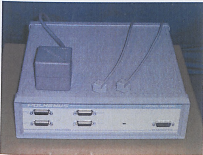
Figure 3.4.2: Fastrak systems electronics unit, TX2 transmitter and two receivers TX2 on the left of picture, receivers on the right
