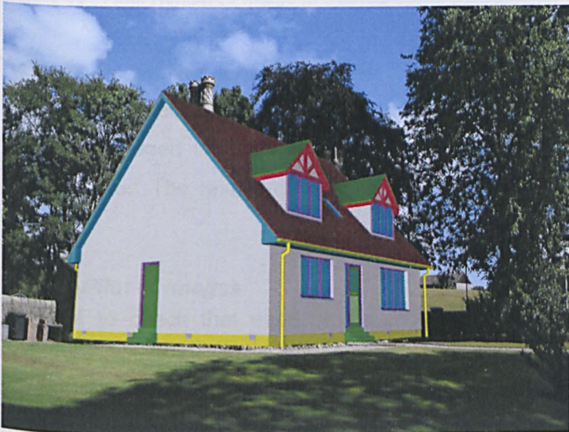
Figure 35 - Lining up the CAD model with the photograph
