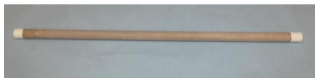
Figure 4: Photograph of the Palladium-coated support
