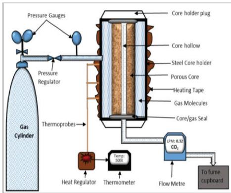
Figure 4 shows the CS experimental pictorial diagram.
