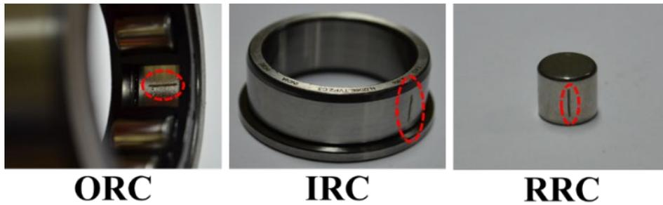
Figure 3: Examples of ORC, IRC, and RRC bearing defects.
