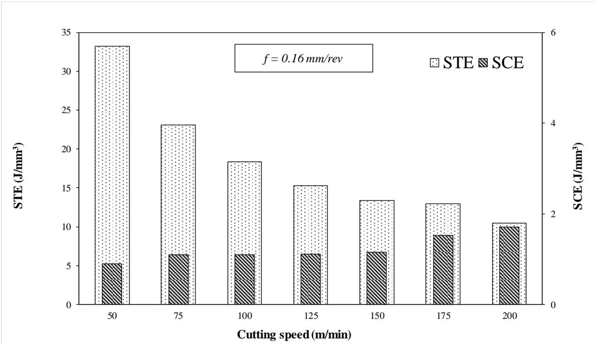
Fig. 9 Trends of Specific Total Energy consumption for machining Ti6Al4V alloy
