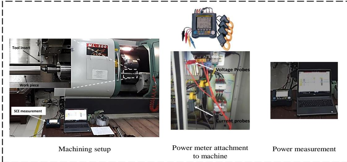
Fig. 4 Experimental setups for measurement of cutting power
