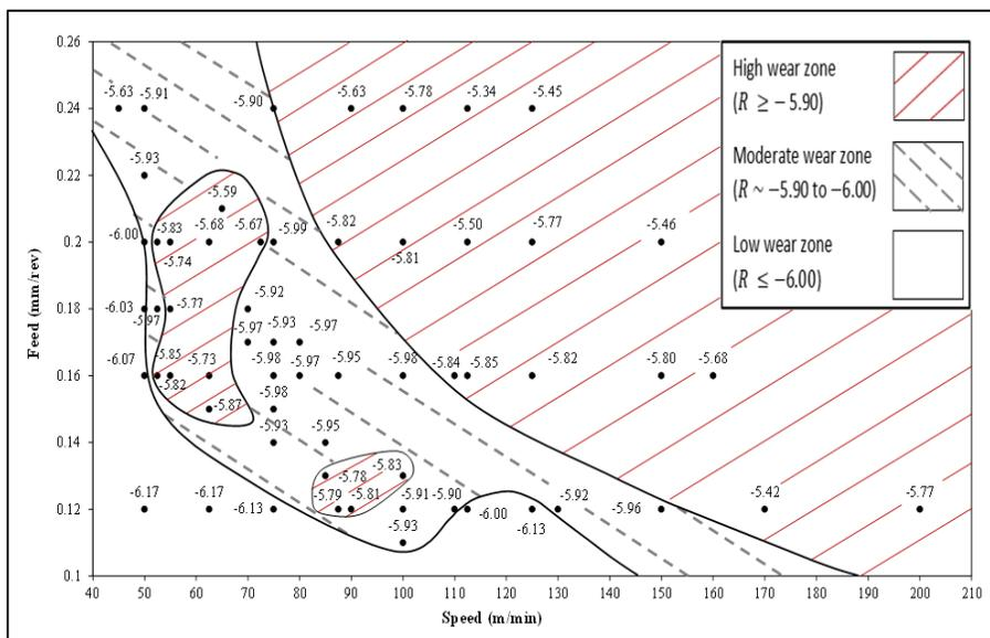
Fig. 7 Map showing wear rate for turning Ti6Al4V
