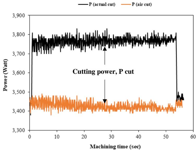
Fig. 5 The energy consumption of the actual cut, and air cut values recorded:  $V = 100$  m/min and  $f = 0.16$  mm/rev.
