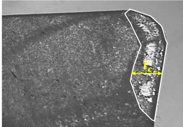
Fig. 6 Measurement of the tool chip contact length
