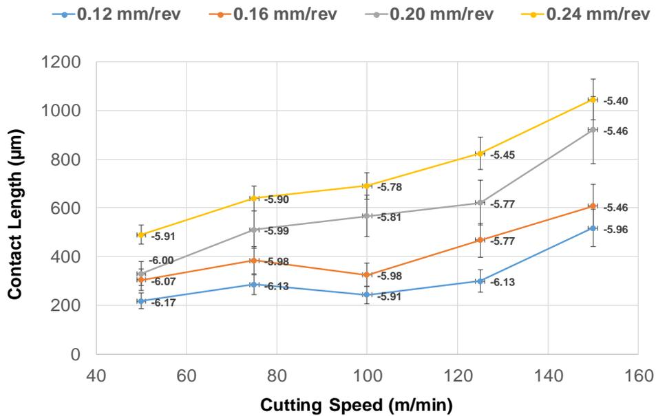
Fig. 10 Influence of the cutting conditions on the contact length
