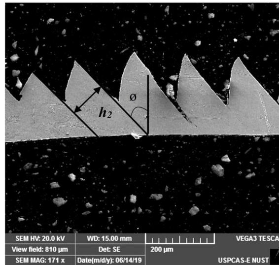
Fig. 11 Micrograph showing the chip segment of Ti6Al4V
