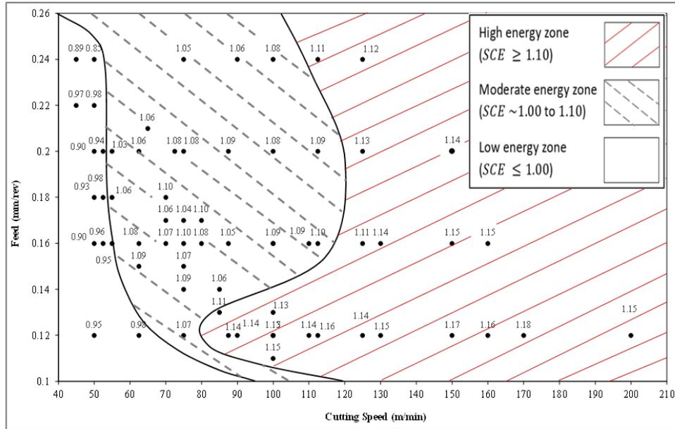
Fig. 8 Map presenting SCE for turning Ti6Al4V
