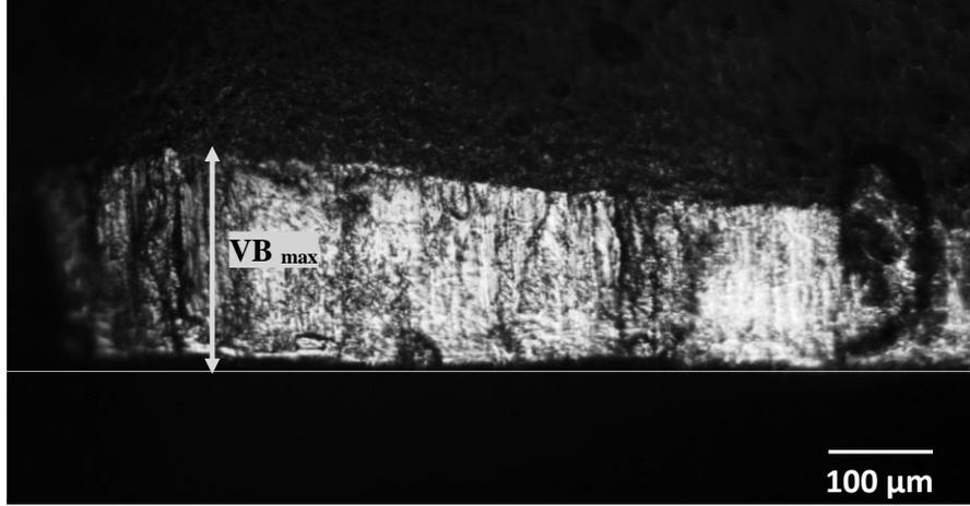
Fig. 3 Optical image showing tool wear land for the measurement of tool flank wear at 20X magnification.
