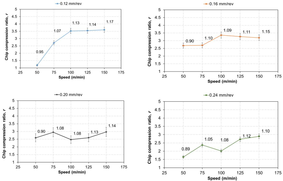
Fig. 12 Chip compression ratio during turning Ti6Al4V at the various cutting combination
