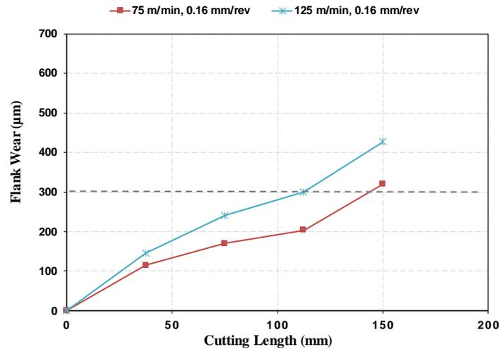
Fig. 2 Trends of wear progression of carbide tool in turning Ti6Al4V alloy
