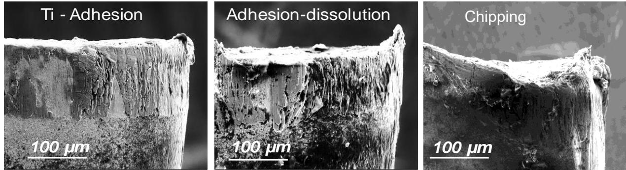
Fig. 15. Tool wear mechanisms in turning Ti-6Al-4V alloy
