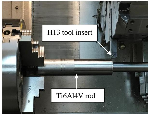
Fig. 1 Turning set-up used for machining
