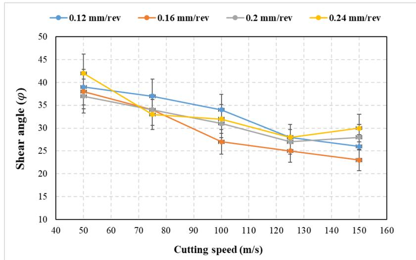
Fig. 14 Experimental shear plane angle ( $\phi$ ) obtained at various cutting speeds
