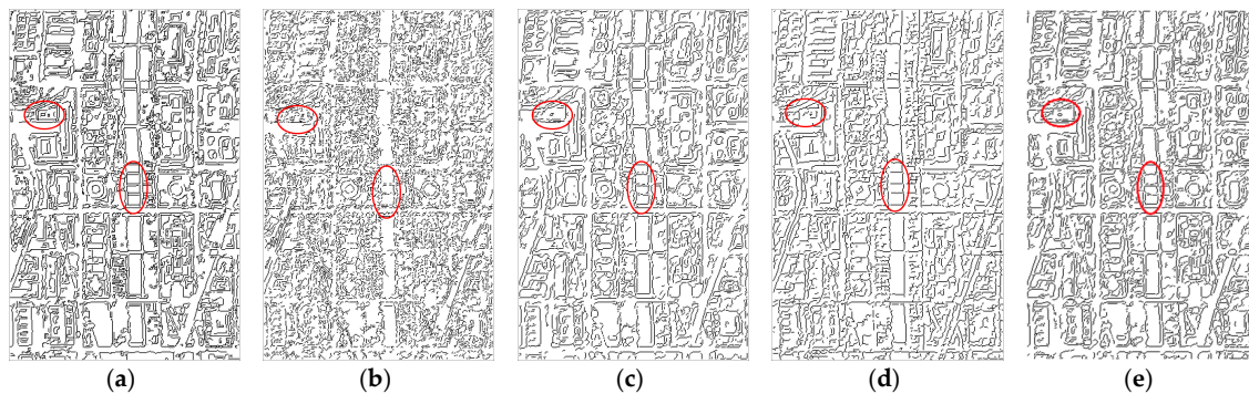
Figure 13. The binary edge maps of the Washington DC Mall by: (a) GEDHSI; (b) Di Zenzo's method; (c) the RCMG method; (d) Drewniok's method ( \sigma = 1.0 ); and (e) SSSDE method.
