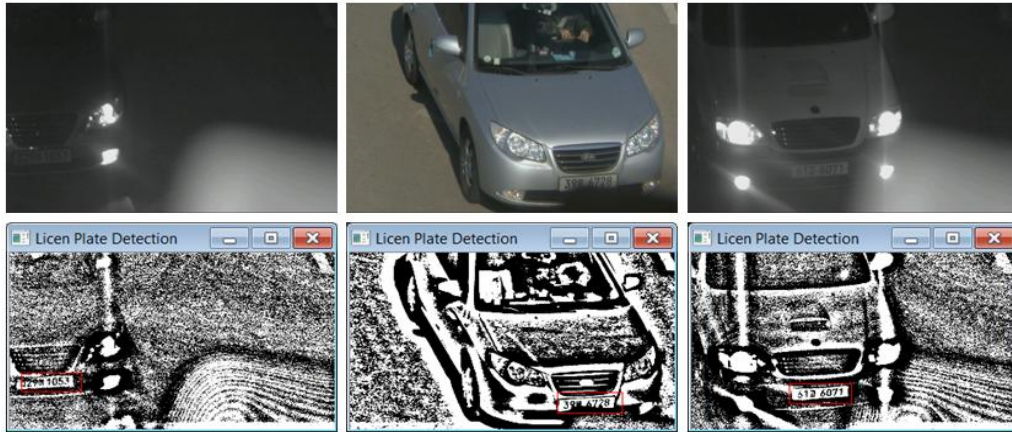
Fig. 16. License plate detection results after applying adaptive thresholding using the integral image
