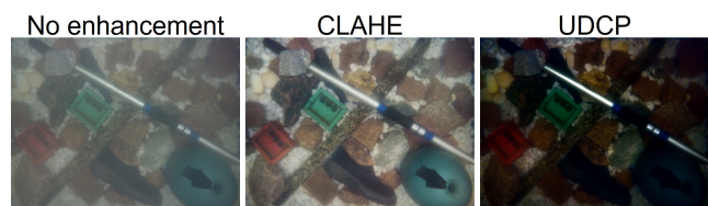
Fig. 4. Comparison of the best and worst UIE methods, CLAHE and UDCP, for one of the original images. In the reconstructed quality scores, CLAHE beats UDCP 16 times (i.e., for all degraded images).
