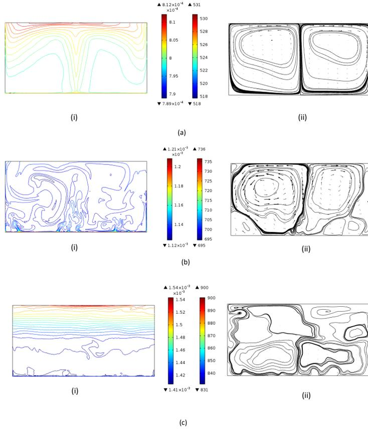
Figure 7: Temperature contours (left) and streamlines (right) for  $H/D=0.5$  (a)  $\tau = 2.27 \times 10^{-5}$  (b)  $\tau = 1.82 \times 10^{-3}$  (c)  $\tau = 3.81 \times 10^{-3}$
