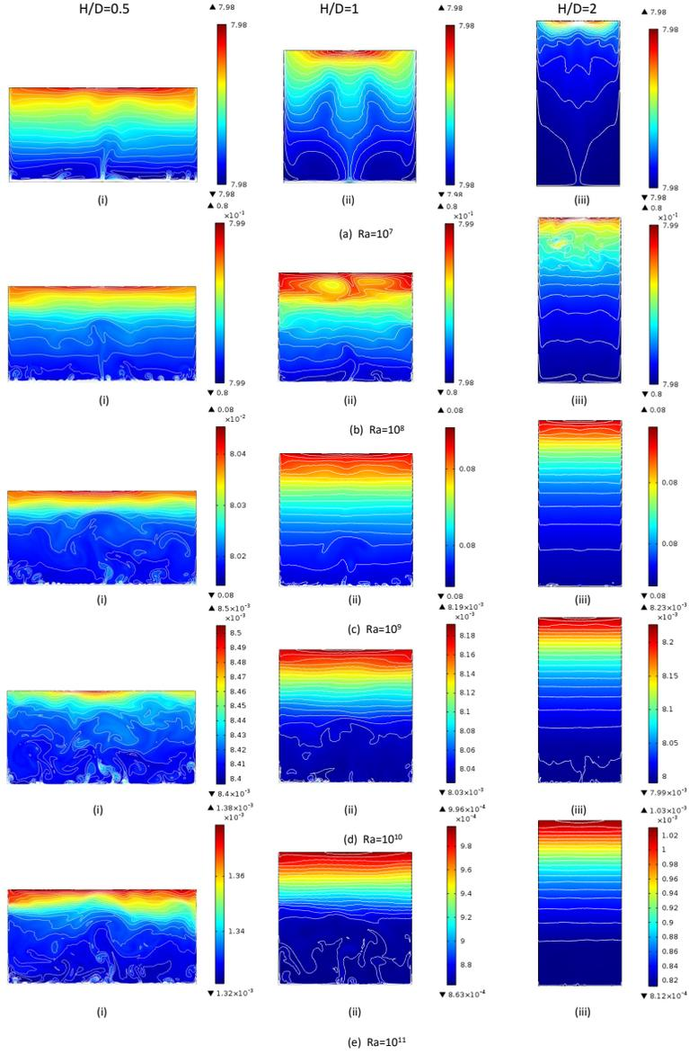
Figure 12: Time averaged temperature contours excluding the quasi steady regime at  $H/D=0.5$  for Rayleigh numbers a)  $Ra=10^7$  b)  $Ra=10^8$  c)  $Ra=10^9$  d)  $Ra=10^{10}$  e)  $Ra=10^{11}$  for  $H/D=0.5$  (left column),  $H/D=1$  (middle column) and  $H/D=2$  (right column)
