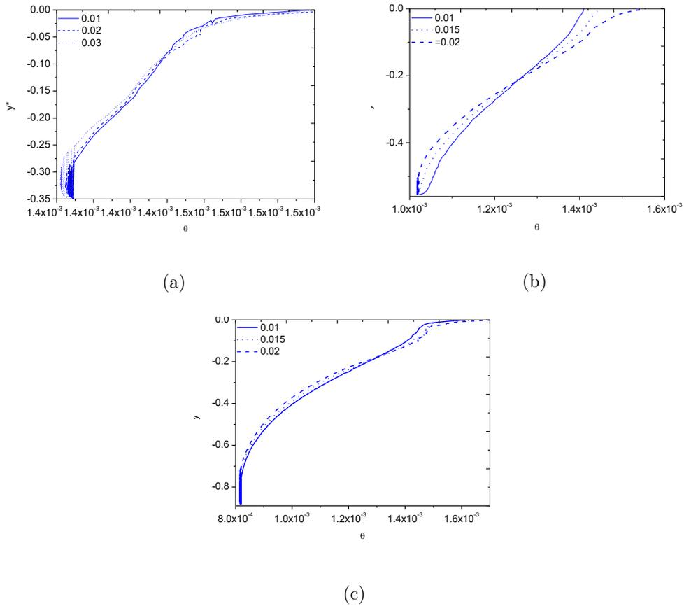
Figure 3: Mesh convergence plot for the temperature taken from the vertical section at  $\tau = 4.5 \times 10^{-3}$  (a)  $H/D=0.5$  (b)  $H/D=1$  (c)  $H/D=2$ .
