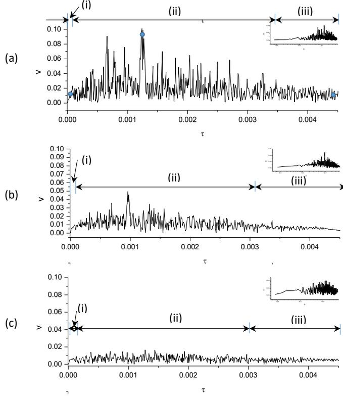
Figure 10: Time series of the flow velocity for  $H/D=0.5, 1$  and  $2$
