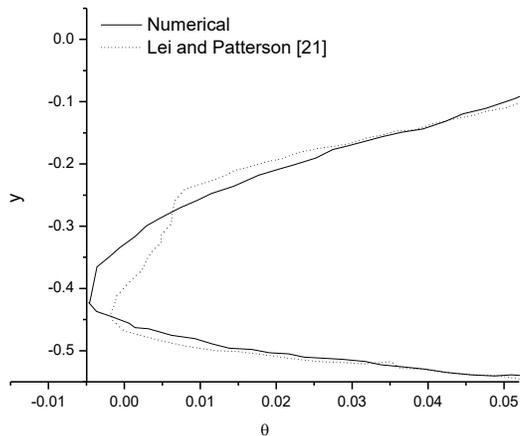
Figure 5: Vertical temperature profile at  $x=5.5$  for experiments (dash) [23] and numerical simulation (solid) at  $\tau = 0.200$  (5049s).
