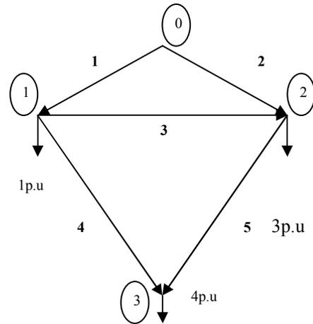
Figure 5 Stochastic network of the three bus system
