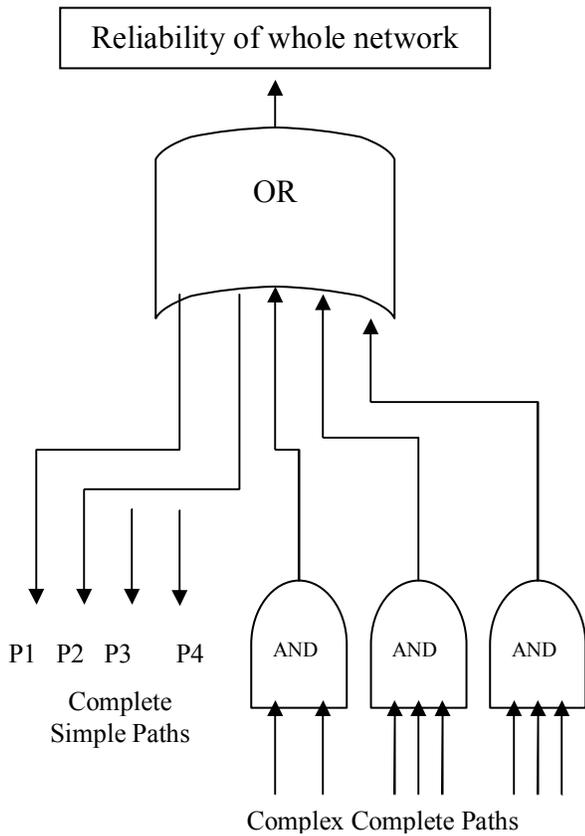
Figure 3 Dual fault tree representation of the whole network
