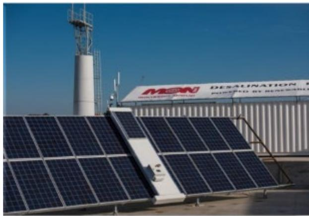
**Figure 14. Dry Panel Cleaning Device [82]**
