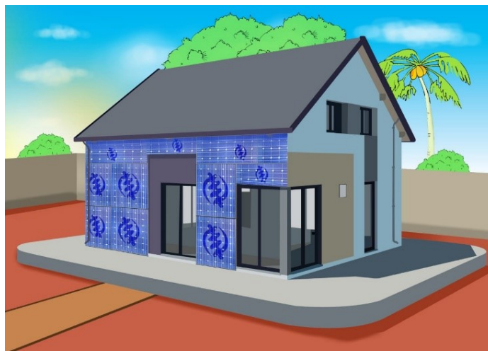
FIGURE 6: An illustration of BIPV building with Adinkra symbols embedded.
