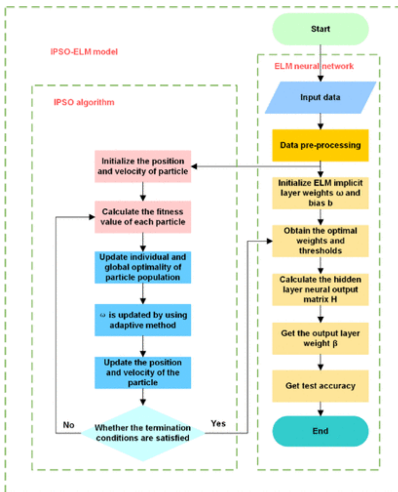
Figure 3. Flowchart of the SOC estimation based on IPSO-ELM.
