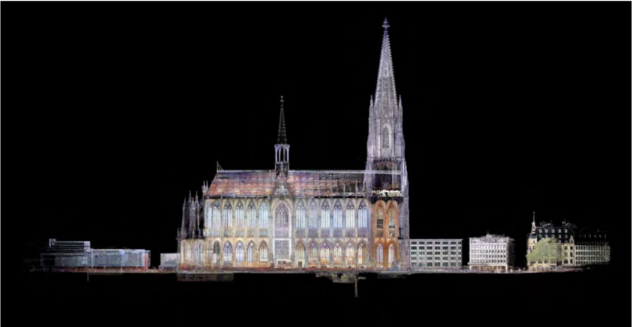
Image 8: Cross-section point cloud rendering through the Cathedral and precinct. Note the foundation tunnel at the base of the tower.
