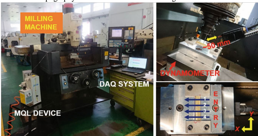
Fig. 2 Machining setup, nozzle distance and cutting path
