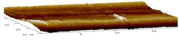
Figure 3.2: AFM image of CDIT Hologram
