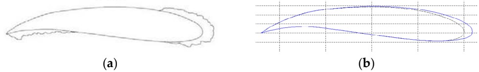
Figure 15. Comparison of ice shapes obtained after 19 min: (a) Experimental shapes obtained by Li et al. [9]; (b) Shape obtained through LewInt.
