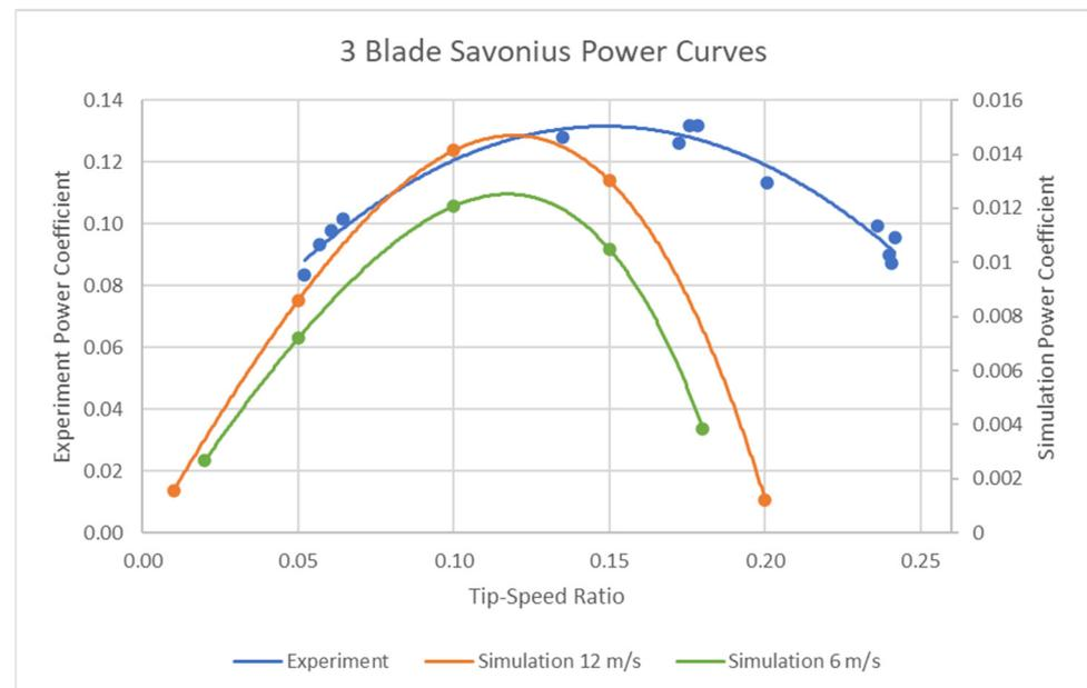
Figure 24. Three-blade Savonius simulation and experiment comparison.
