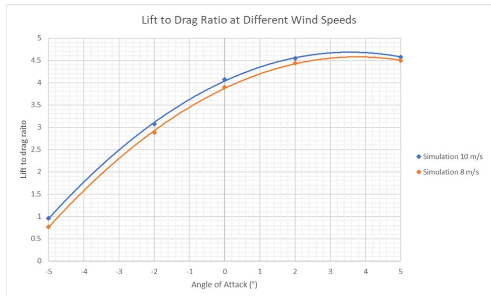
**Figure 7.** Single blade lift to drag ratio.
