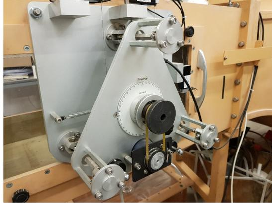
**Figure 5.** Three-point balance.
